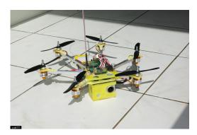
W. Thielicke shows his ne shrediquette MM6 on his <a href="https://homepage">homepage</a>, which was designed to carry the GoPro HD camera. This copter should be a reliable and solid platform for fpv flying. I liked the design so much and after i saw his
